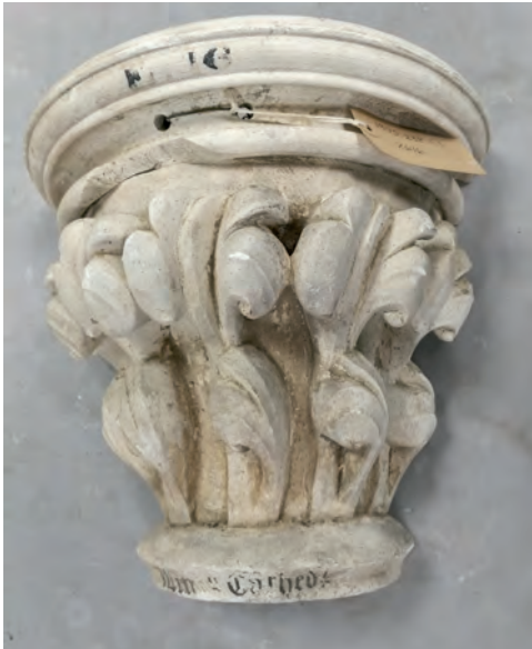
Fig. 4. Cast of capital (Early English) from Lincoln Presbytery with crisp detail from a plaster piece-mould, the damage to abacus showing cast in two or more lifts (OAS-E16/OMS-1975.238.43).
