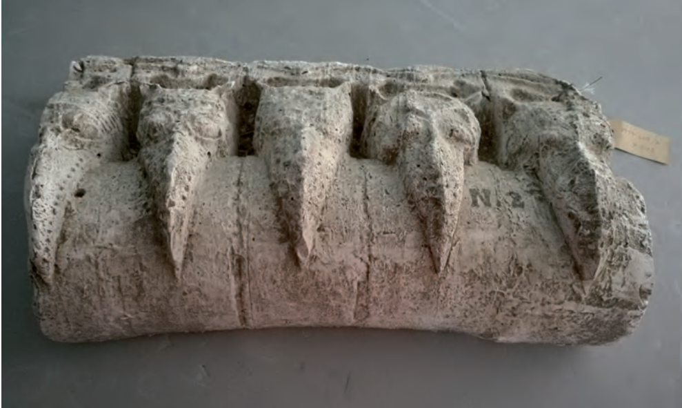
Fig. 7. Section of moulding with beakhead decoration taken from west door of Iffley church. Note porous casting, possibly using clay mould. Almost certainly work of T. Grimsley (OMS-N2/OMS-1975.238.2).
