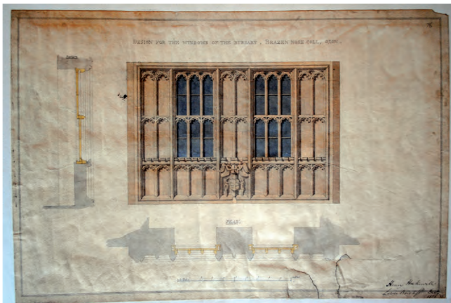
Fig. 11. Henry Hakewill, 'Design for the windows of the Bursary, Brazen Nose Coll. Oxon.' (Dec. 1816), plan, section and elevation in ink and wash. Brasenose College Archive, with permission the principal and fellows of Brasenose College.
