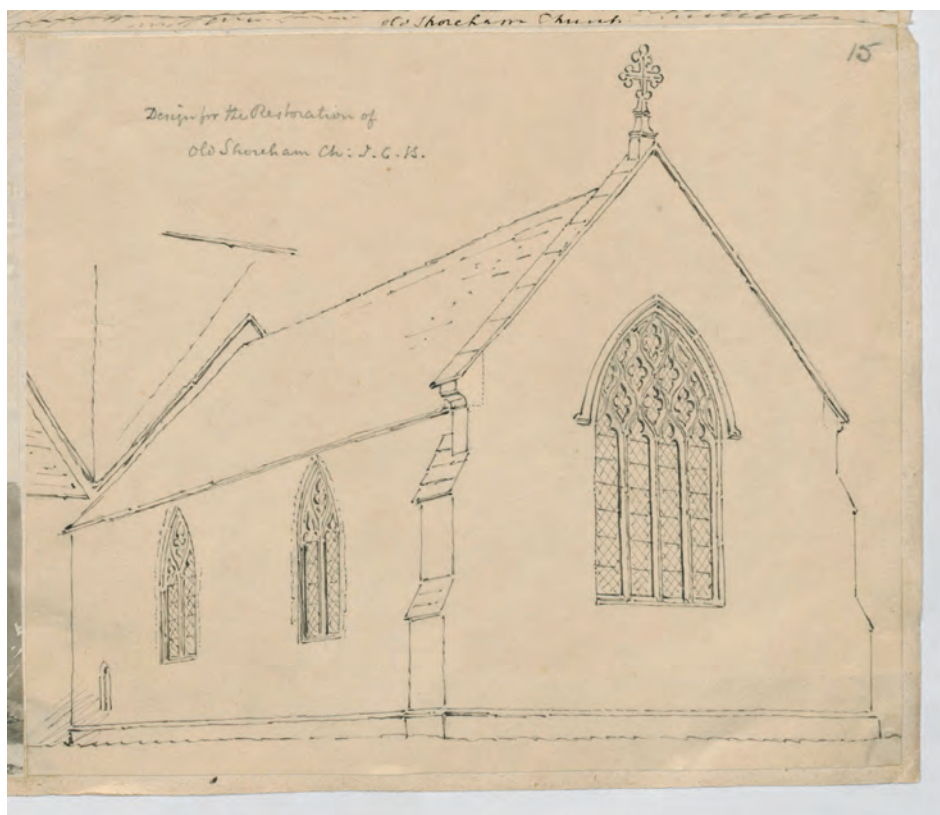
Figs. 3 and 4. J.C. Buckler's sketches of extant condition and projected restoration at the church of St Nicholas, Old Shoreham (1839). BL, Add MS 36443, ff. 13, 15.
