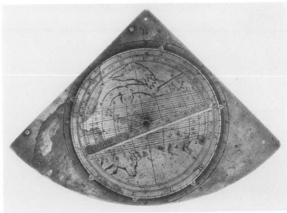
Fig. 3. Horary quadrant, brass. Signed: I. * P. Fecit Oxō. 103.5 mm. radius. Face a (Top): Gunter projection [for a latitude of about 51° 45']. Face b (Bottom): Planispheric nocturnal and analemma. Museum of the History of Science, Oxford, 86-8.
