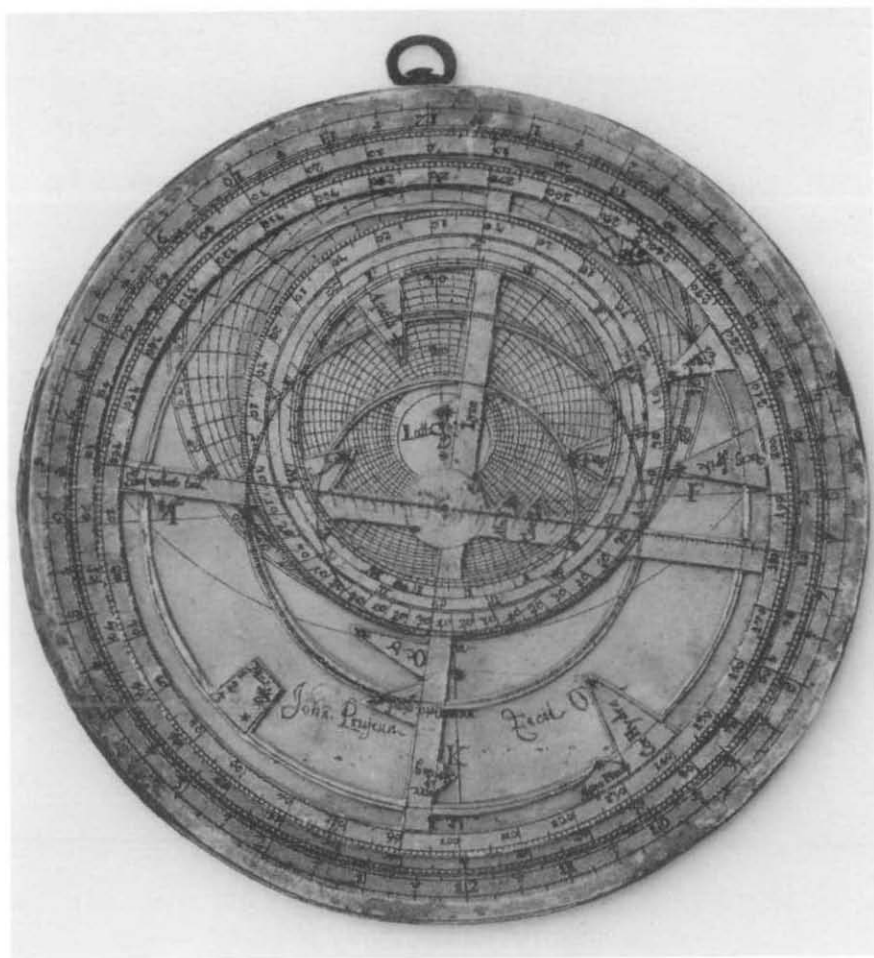
Fig. 4. Astrolabe to the design of Thomas Edwards, engraved paper, on wood and card. Signed on the latitude plate for 51^{\circ} 45' : Joh. Prujean Fecit Oxon 203 mm. diameter. Museum of the History of Science, Oxford, Lewis Evans Collection 2094, IC 314.
