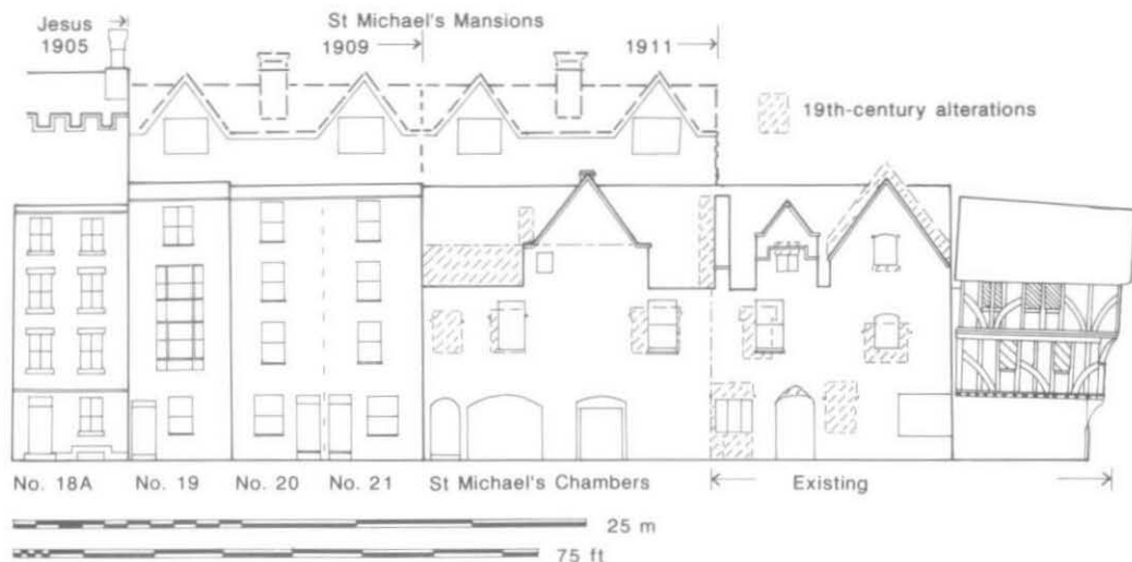
Fig. 9. Ship Street elevation: composite view showing exterior of north range (with alterations) and adjacent houses, with outline of Jesus College buildings (from photographs, Parker drawing and as existing).
