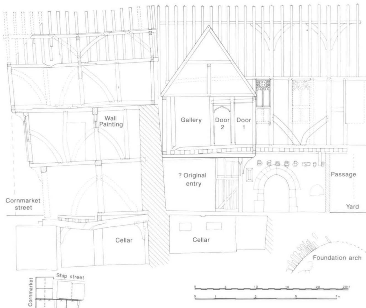
Fig. 13. The New Inn, 1984: section looking north through Cornmarket shops, gallery and cellars, with south elevation of north range. (N. Joyce and OAU).
