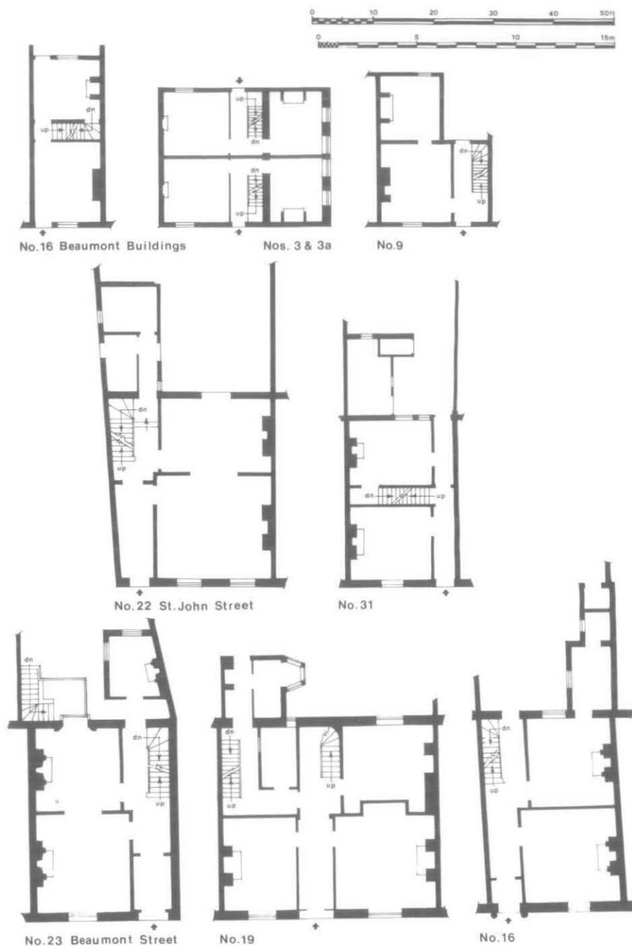
Fig. 2. Houses in St. John Street, Beaumont Street and Beaumont Buildings: specimen ground-plans. (Re-drawn, with amendments, from architects' plans provided by Messrs. Cluttons.)
